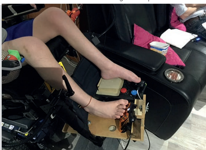
The joystick was removed from the controller and placed near his left foot for ease
