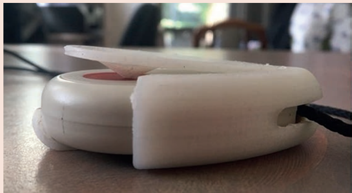
A 3D printed cover to help with pressing the button on a personal alarm completed by Rob
